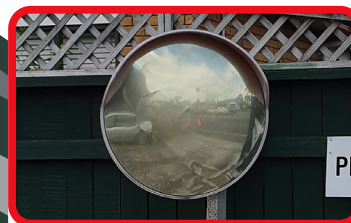
Visible Crazing, Yellowing and Delamination
