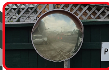
Visible Crazing, Yellowing and Delamination
